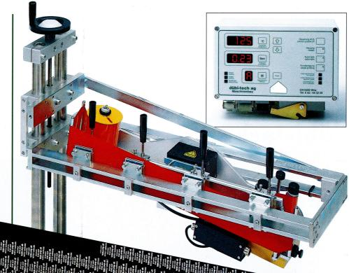
With the Multi-Printer there can be used clichées, steel types and datingsystems. Any of these printing tools can be combined.
